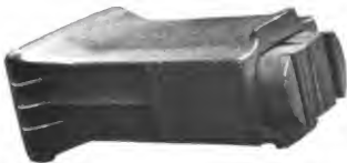
Fig. 3961. Gould Friction Draft Gear, Assembled.
